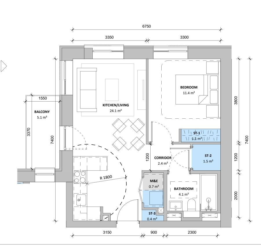
All dimensions to be checked on site. Figured dimensions take preference over scaled dimensions. Any errors or descrepancies to be reported to the Architects. This drawing may not be edited or modified by the recipient.
